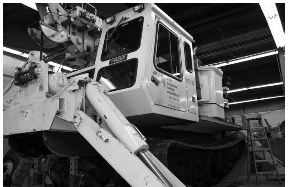
This beast, with tracks instead of wheels and a variety of mechanized outriggers, will come in handy for stringing wire in the refurbished right-of-way in Chelsea.
