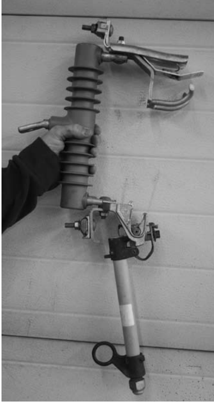
Visual aids help the Co-op's line workers find the source of an outage more quickly. Fuses (above) are linked to the lines, and when a fault occurs and blows the fuse, the door drops open (left). That provides a clue to the location of the outage; blown fuses must be replaced. A Trip Fault Indicator (right) can tell a repair crew whether the fault is ahead of them or behind them, depending what color shows in the bubble at the bottom. No replacement necessary here.
